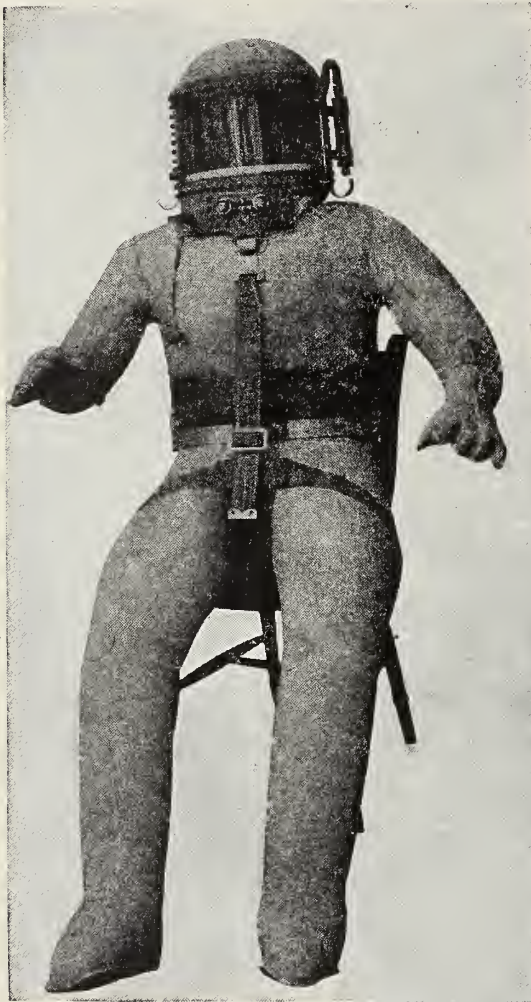
Fig. 27. Two pictures of the British Royal Air Force oxygen-pressure suit that was used in breaking the world's airplane record for high altitude
